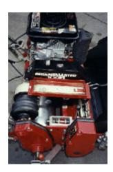
The frame is made of 1" angle iron with tabs to attach it to the drive belt housing. It's mounted on a spot where it doesn't seem to effect the balance of the machine, although it does add some weight. It's held on with a bungee cord, and when not in use, it can easily be taken off
